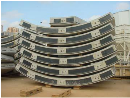
Figure 7. Iron-concrete segments constructed for a metro installation (a) and its test (b) [13].
