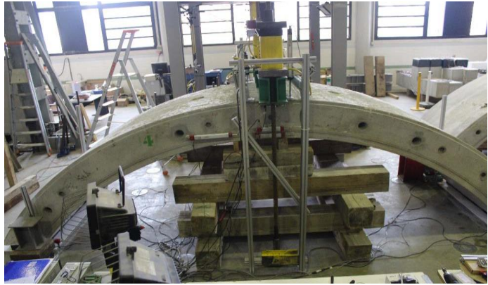
Figure 7. Iron-concrete segments constructed for a metro installation (a) and its test (b) [13].
