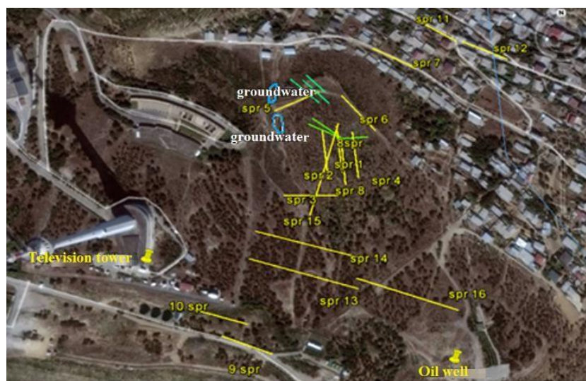
Fig. 3. Scheme of seismic profiles in the study area (16 different profiles developed)
