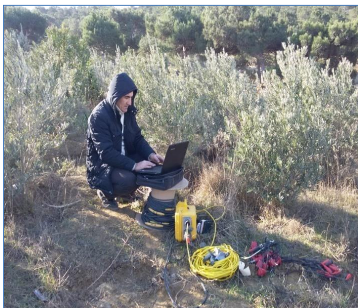
Fig. 8. Placement of seismic receivers on the profiles of the study area and registration of seismic waves
