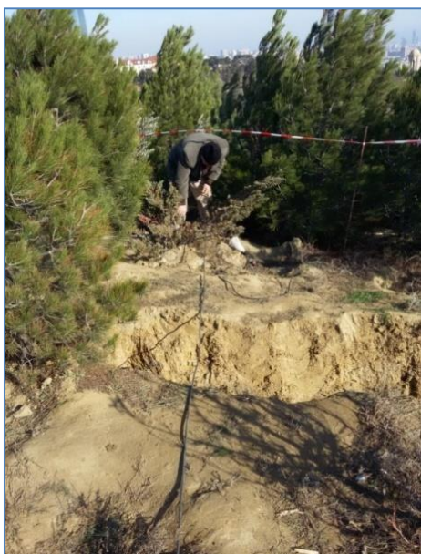
Fig. 8. Placement of seismic receivers on the profiles of the study area and registration of seismic waves
