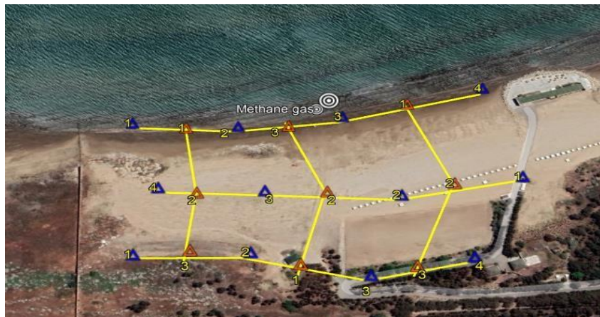
Fig. 2. Scheme of gravimetric observation points carried out in the study area Symbols:
