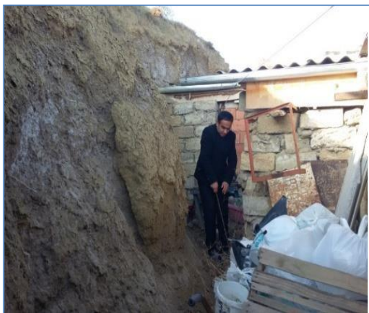
Fig. 6. Slope cut in front of the landslide zone and rock sampling from a shallow depth
