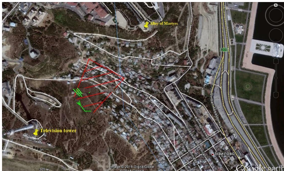
Fig. 1. General view of the landslide with observed main fractures in the area
