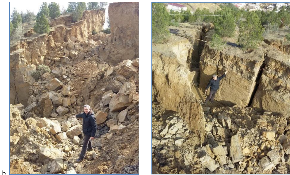
Fig. 15. Terrain change observed at a depth of about 10 m at a distance of 19 m at the top of the landslide
