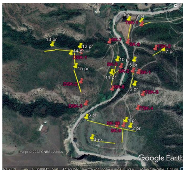
Figure 4. Location scheme of 15 seismic profiles in the research area. Symbols: SK, DSK, TSK – red signs - exploration holes, yellow signs - seismic profiles.
